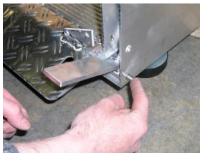
1. Loosen screw on remote control side and sink in side rail to assemble side part (for later screw-connection).
