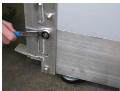
3. Assembly of side parts: - with 7 screws 10 x 60 + nuts; each rail 2 pieces to upper drill-holes; Exception: side with remote control pedal , this side up only 1 screw - and 3 screws 10 x 80 + nuts; each rail 1 piece to lowest drill-hole; Exception: side with remote control opening no screw at bottom
