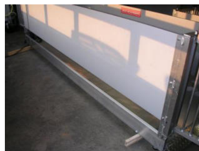
2. Insert evenly into side rail of base plate.
