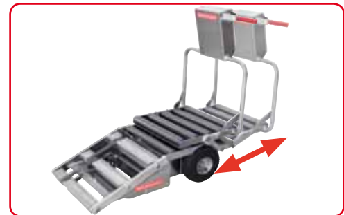
Foldable loading table for working in confined spaces. The user takes the vehicle in retracted state to the animal. The loading table unfolds while pulling the animal onto the vehicle.
