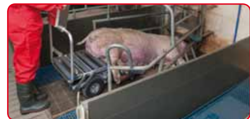
Foldable loading table for working in confined spaces. The user takes the vehicle in retracted state to the animal. The loading table unfolds while pulling the animal onto the vehicle.
