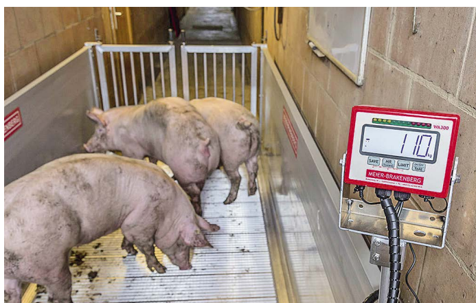
For so-called ‘zero weighing’ all animals of a group are driven onto the deck. Then each animal leaves the deck one at a time. As each leaves, its weight is indicated marked by a minus sign. The software has meanwhile been reprogrammed so the ‘traffic light’ system also works for negative readings.
