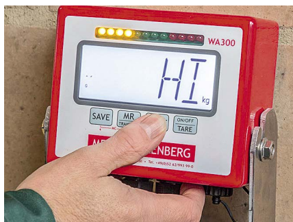
You enter three weight ranges to customise the traffic light system to your needs.
