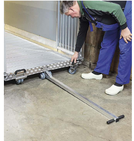
The low-floor weighing machine runs on idler wheels that are fitted without tools.
