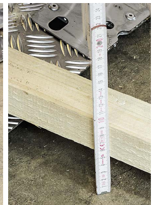
The low-floor weighing machine boasts a weighing deck that's only 5cm off the ground (right). This in conjunction with an aluminium ramp has reduced the step-on height to 2cm. So wheeled equipment - even on small wheels - can overcome the weighing platform, which eliminates the need of embedding it in the floor.
